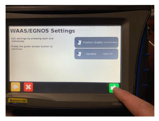
10)You may need to save your configuration when you are finished. If you have multiple configurations saved in the display, you will need to load each configuration, make the GPS setting change, and then save/overwirte the old configuration.
