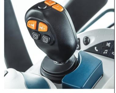
The joystick returns to the center, neutral position when released, except when it is in float position.
